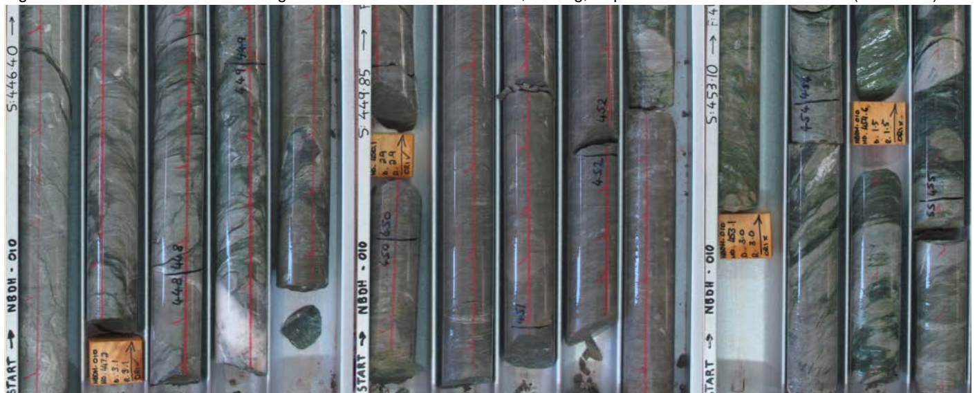
Figure 3 – NBDH010 drillcore showing shear zone related deformation, veining, sulphidation and fuchsite alteration (446-456m).
