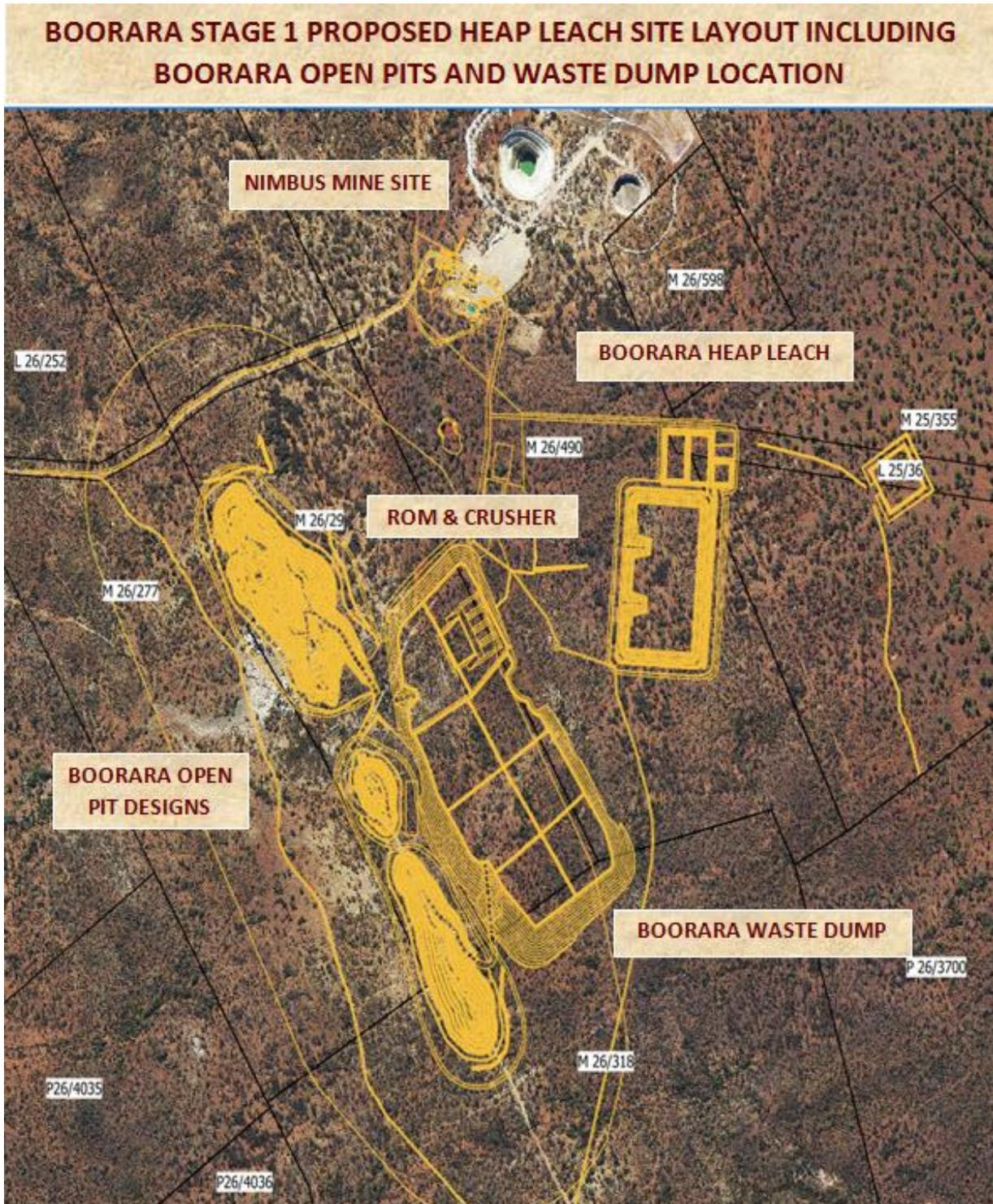
Figure 2: Boorara Stage 1 proposed site layout.
